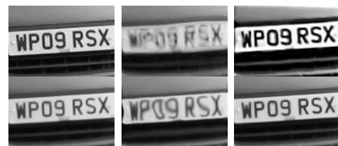
Fig. 1. Image restoration. From top to bottom: the ground-truth image, the distorted and blurred image, the Sobolev gradient-Laplacian method [189], the centroid method [202] deblurred [259], the two-stage reconstruction method [213] and the RPCA algorithm [154]. (Images from [154].)
