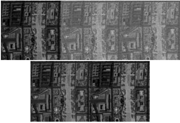
Fig. 3. Hyperspectral image denoising results of band 100 for Washington DC Mall data set. From top to bottom: original band, noisy band, the wavelet-based result, GoDec [350], and RPCA algorithm [296]. (Images from [296].)
